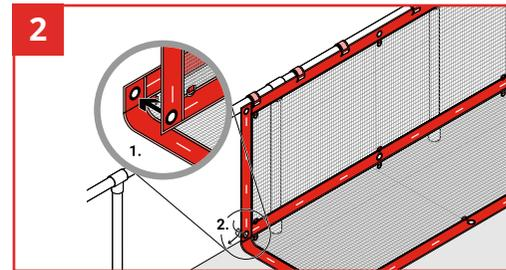
To combine multiple Gap Guard together, overlap Velcro edging of each Gap Guard. Ensure no kinks or gaps exist. Once overlapped, add further security by securing ties through the perimeter eyelets.
