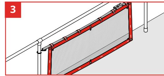
To secure Gap Guard on ratchet straps, attach in the same manner as step one.
