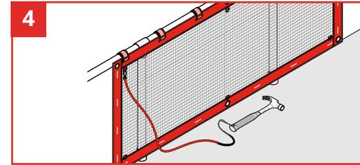
Attach GRIPPS® tool tethers to D-ring anchor points as necessary. Never exceed maximum load. Always be cautious of maximum tether length.
