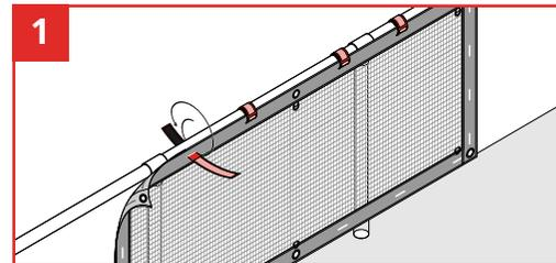
Position Gap Guard against handrail or flooring. Secure Velcro straps to handrail or grid mesh around the perimeter of Gap Guard evenly.
