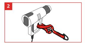
Pass one end of the Tool Hitch around the neck (near the tool's center of gravity). Then pass the D-Ring end back through the Tool Hitch loop to create a choke-hold.
